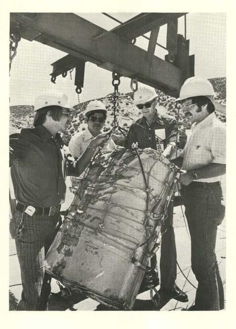
PLUTONIUM ACCIDENT RESISTANT CONTAINER developed by John Andersen (3rd from left, 5433) is shown before accelerated impact test, one of a series. After test, outside shell of container was badly damaged but inside cannister was intact. Bryan Joseph (5432), Mike Huerta (1282) and Mike Stone (5431) helped John in various aspects of container development.
